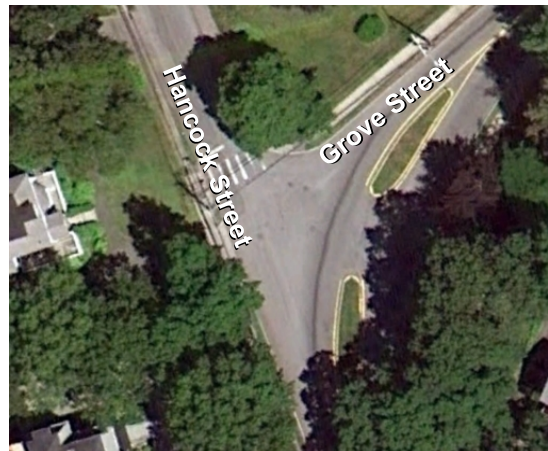
Grove Street at Hancock Street: skewed “T” intersection with no demarcation of turning movements
