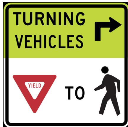
FIGURE 2 MUTCD Sign R10-15: Turning Vehicles Must Yield to Pedestrians
