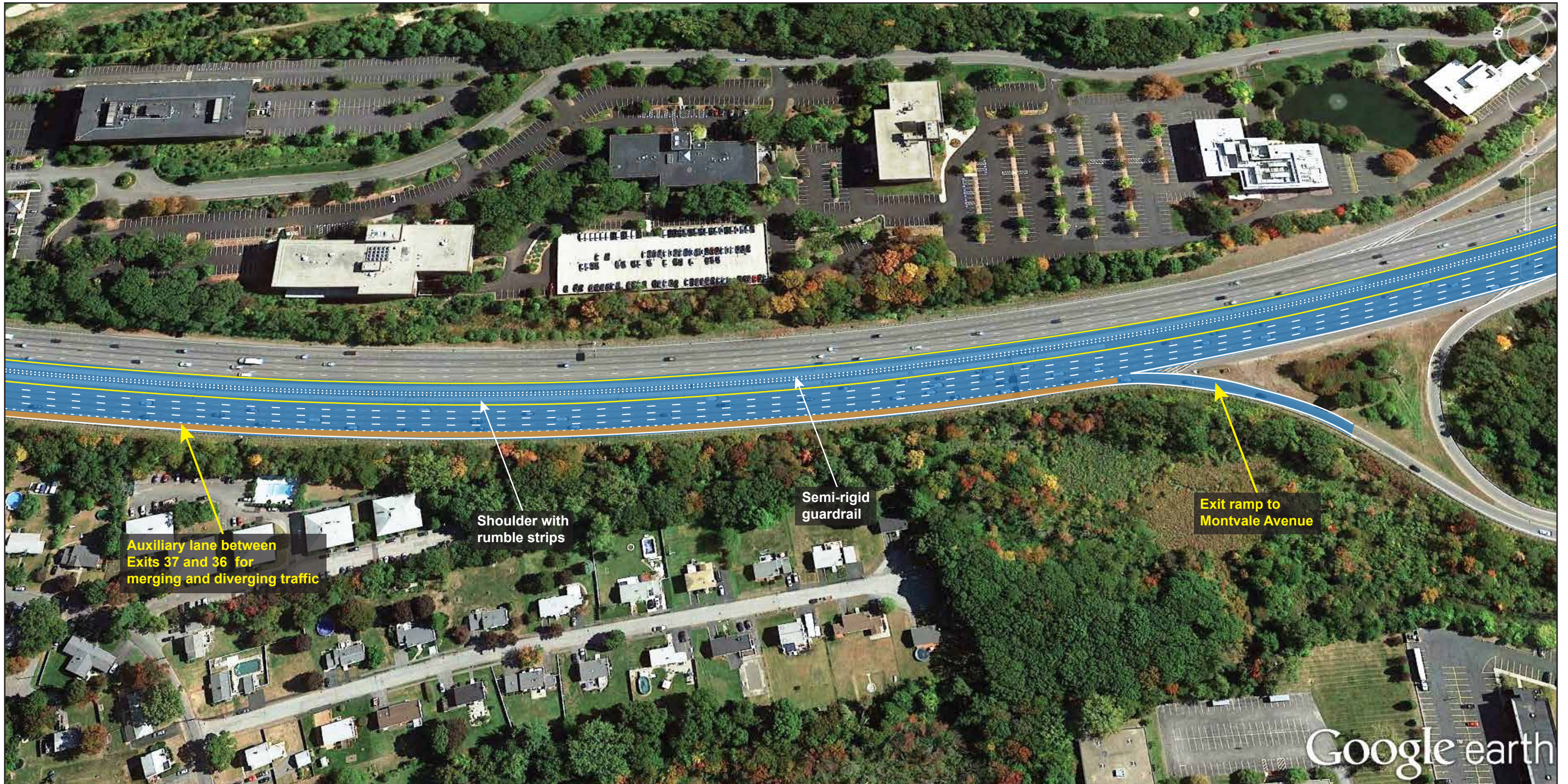
FIGURE 7 (Section 3) I-93 Southbound Segment: Between I-95 and Montvale Avenue Alternative 2: Construct an Auxiliary Lane Using Existing Right Shoulder
