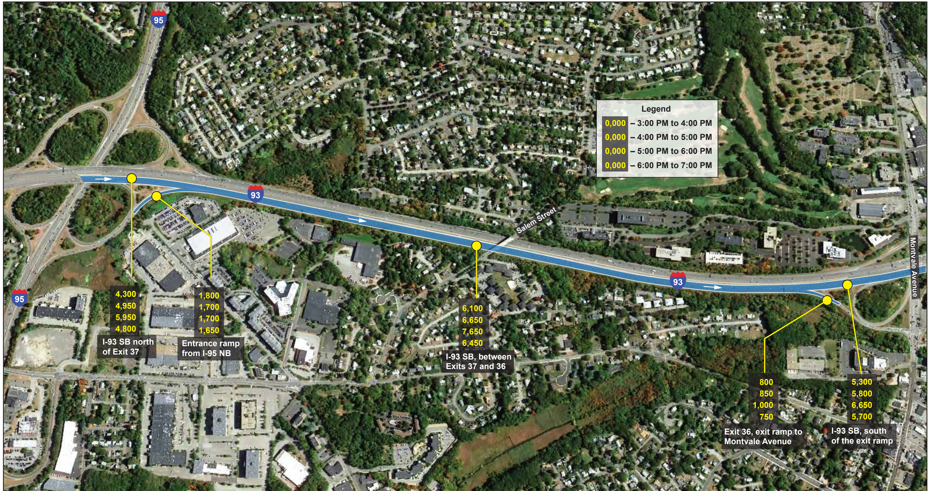
FIGURE 3 I-93 Southbound Segment: Between I-95 and Montvale Avenue PM Peak Period Balanced Traffic Volumes
