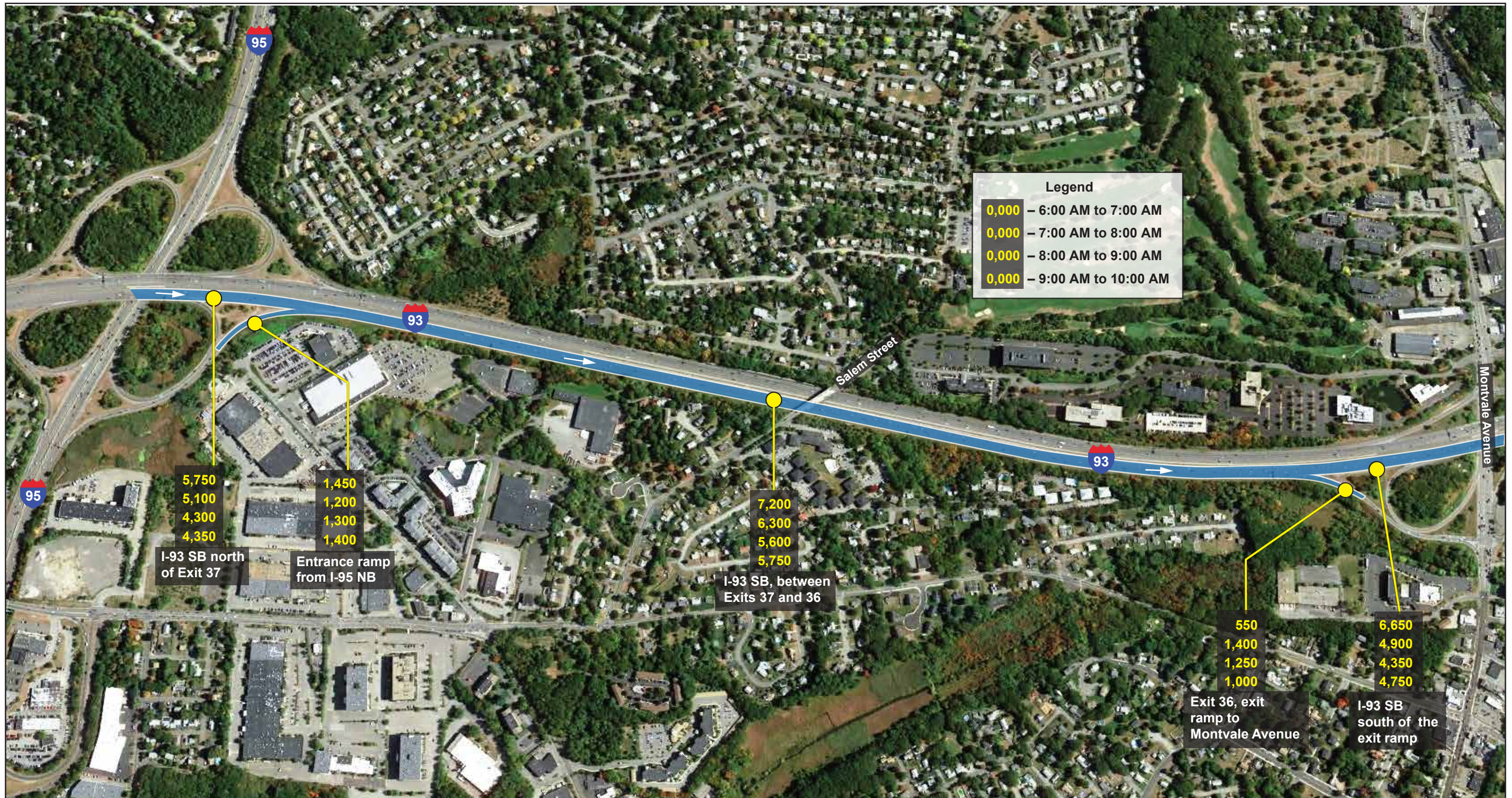
FIGURE 2 I-93 Southbound Segment: Between I-95 and Montvale Avenue AM Peak Period Balanced Traffic Volumes
