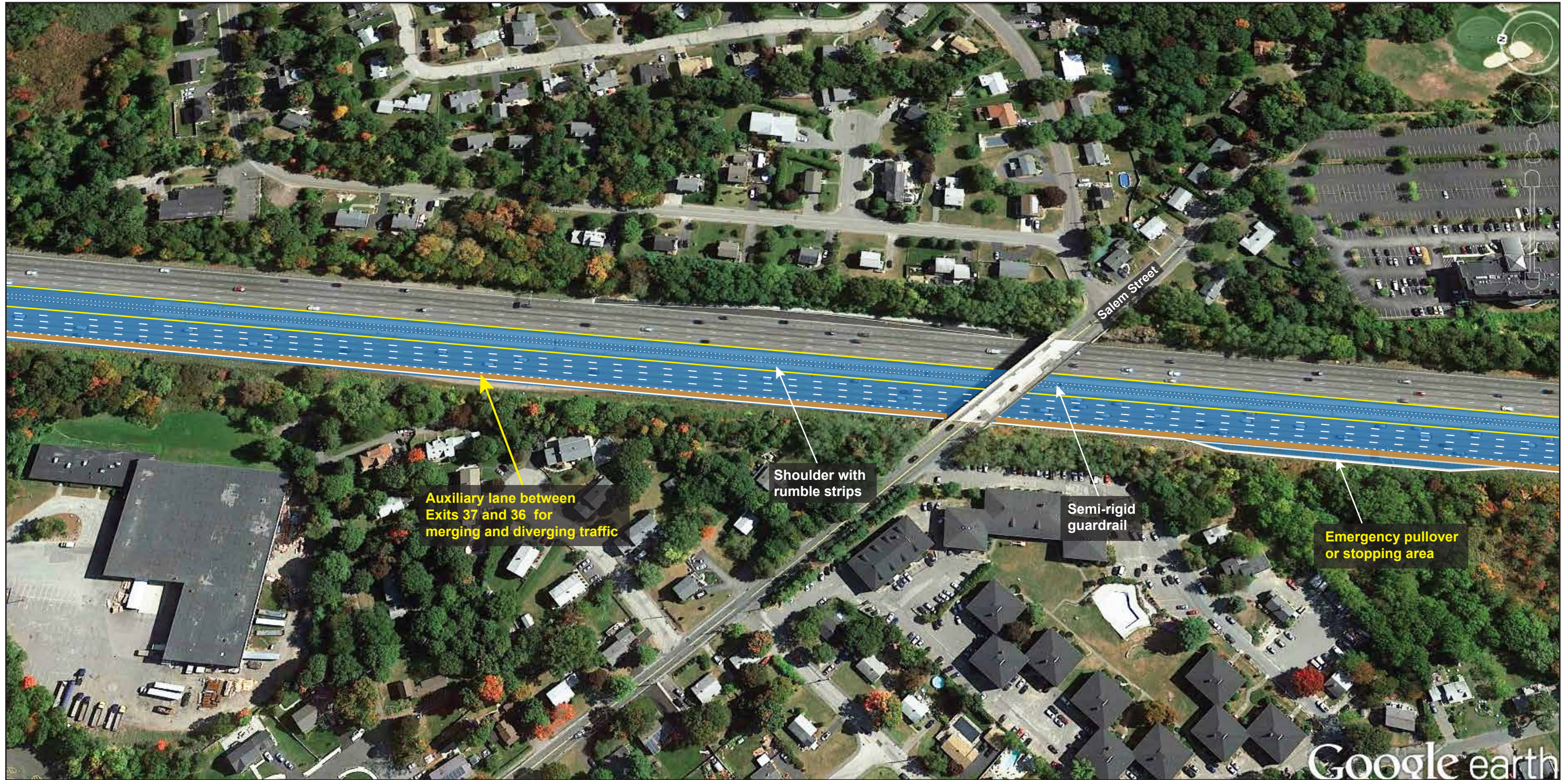
FIGURE 7 (Section 2) I-93 Southbound Segment: Between I-95 and Montvale Avenue Alternative 2: Construct an Auxiliary Lane Using Existing Right Shoulder
