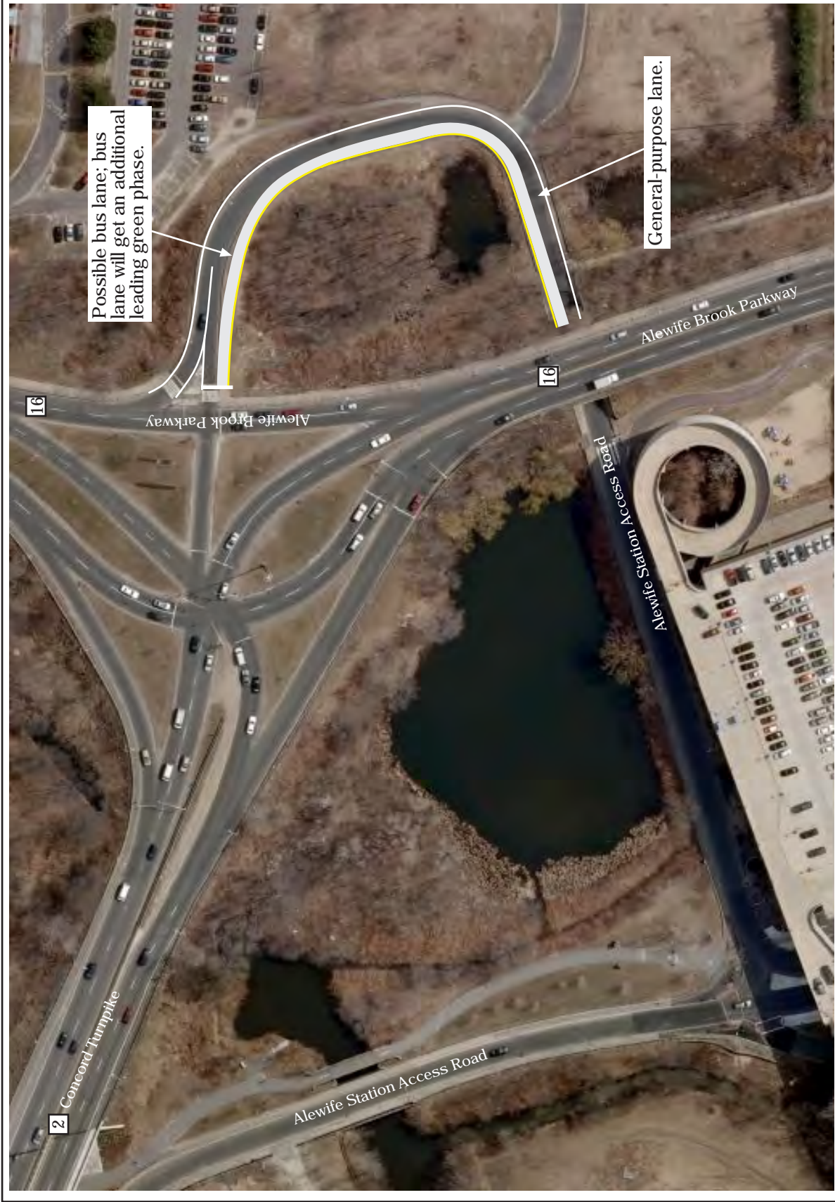
FIGURE 12 Widen Alewife Station Access Road (Jug-handle) to Two Lanes and Install Bus Priority
