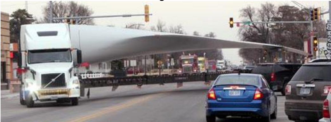
Figure 11 Oversized Loads: Delivering a Wind Turbine Blade
