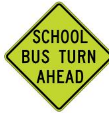
Figure 11c Recommended “School Bus Turn Ahead” (S3-2) Sign
