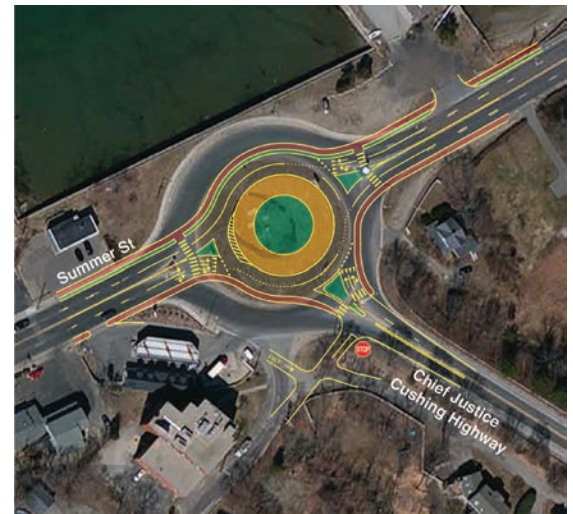
An MPO study has proposed two alternatives for replacing the Route 3A rotary in Hingham. The overlays above show the layout of a proposed signalized intersection (left) and a modern roundabout (right) over the existing rotary. [Photo: GoogleEarth]
