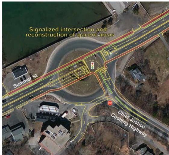
An MPO study has proposed two alternatives for replacing the Route 3A rotary in Hingham. The overlays above show the layout of a proposed signalized intersection (left) and a modern roundabout (right) over the existing rotary. [Photo: GoogleEarth]
